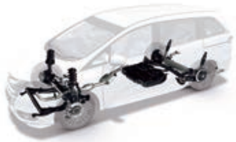
超薄型のPFTはオデッセイの低床・低重心に大きく寄与 Super thin PFT contributes greatly to the Odyssey's low floor and low center of gravity
